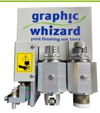
Dual RCT : **Rotary Cutting Tools** cuts up to 1.8mm
